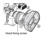
To reattach the hood, align the marks on the hood with those on the camcorder, turn it in the opposite direction from that when you removed it, then tighten the fixing screw.
